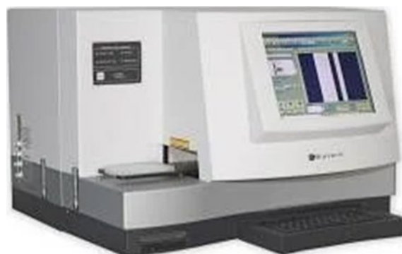
Fig 7. Commercial instrument of electrochemiluminescence M-SERIES ® 384 Analyzer by BioVeris Corporation [73]
