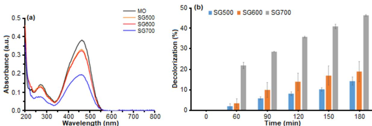
Fig 7. (a) UV-Vis Spectra of MO photocatalyzed for 180 min; (b) Decolorization percentages of MO dye
