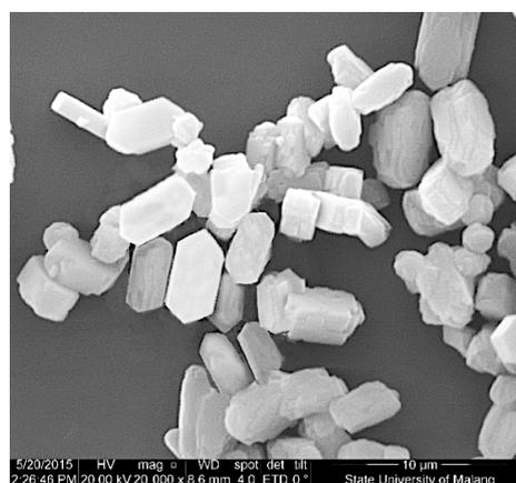
Fig 3. Micrograph SEM of synthesized ZSM-5
