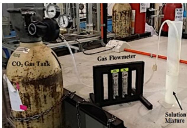
**Fig 1.** Experimental setup of the foam stability at static bulk scale with the gas flow controller for air flow control
