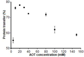
**Fig 4.** Effect of AOT concentration on protein recovery during forward extraction. Experiment conditions: NaCl concentration=0.1 M; pH = 5, volume of organic to aqueous phase = 1:1, contact time = 15 min
