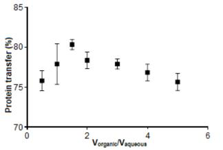
**Fig 5.** Effect of volume ratio of organic phase to aqueous phase during forward extraction. Experiment conditions: NaCl concentration=0.1 M; pH = 5, AOT concentration = 20 mM, contact time = 15 min
