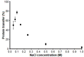
**Fig 2.** Effect of NaCl concentration on protein recovery during forward extraction. Experiment conditions: pH = 5; AOT concentration = 20 mM, volume of organic to aqueous phase = 1:1, contact time = 20 min
