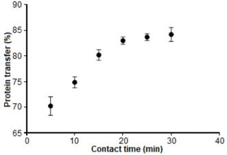
**Fig 6.** Effect of contact time during forward extraction. Experiment conditions: NaCl concentration=0.1 M; pH = 5, AOT concentration = 20 mM,  $V_{org}/V_{aq} = 1:1$
