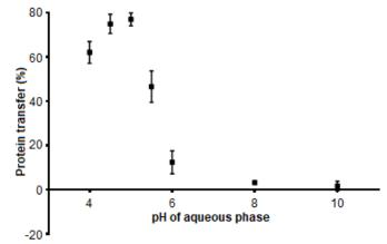
**Fig 3.** Effect of aqueous phase pH on protein recovery during forward extraction. Experiment conditions: NaCl concentration = 0.1 M; AOT concentration = 20 mM, volume of organic to aqueous phase = 1:1, contact time = 15 min
