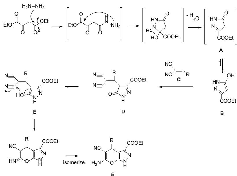
Scheme 2. Plausible mechanism for the synthesis of 5(a-t)
