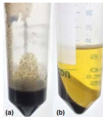
Fig 7. The mixture of rice husk and products after the reaction, using: (a) \text{MnCl}_2 \cdot \text{H}_2\text{O} and (b) MnOx/Hi_ZSM-5 as a catalyst
