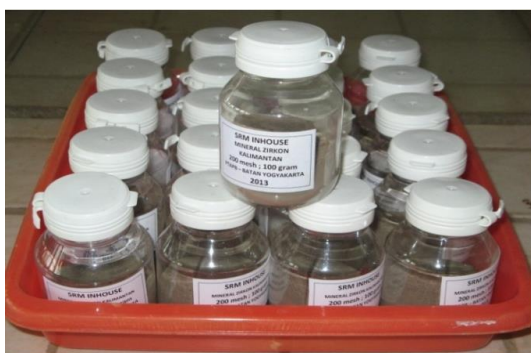
Fig 2. The powder of standard reference materials (in-house) zirconium minerals from Kalimantan passes 200 mesh, number of 40 bottles, packs of 100 g
