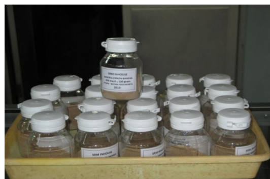
Fig 3. The powder of standard reference materials (in-house) zirconium minerals from Bangka passes 200 mesh, number of 40 bottles, packs of 100 g
