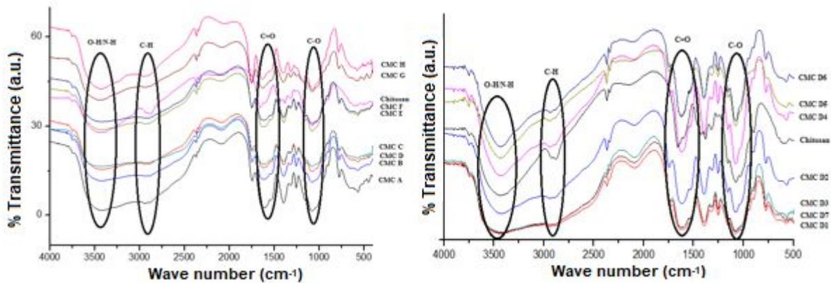
Fig 6. FTIR spectra of chitosan and CMC varied by temperature and varied by NaOH concentration
