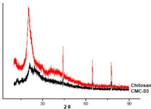
Fig 7. XRD diffractogram of chitosan and CMC-D3
