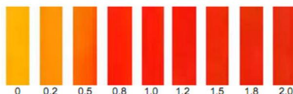
**Fig 7.** Color change of the sensor membranes in 2 mL Cd(II) solution at concentration the range of 0-2 ppm and pH 8.0
