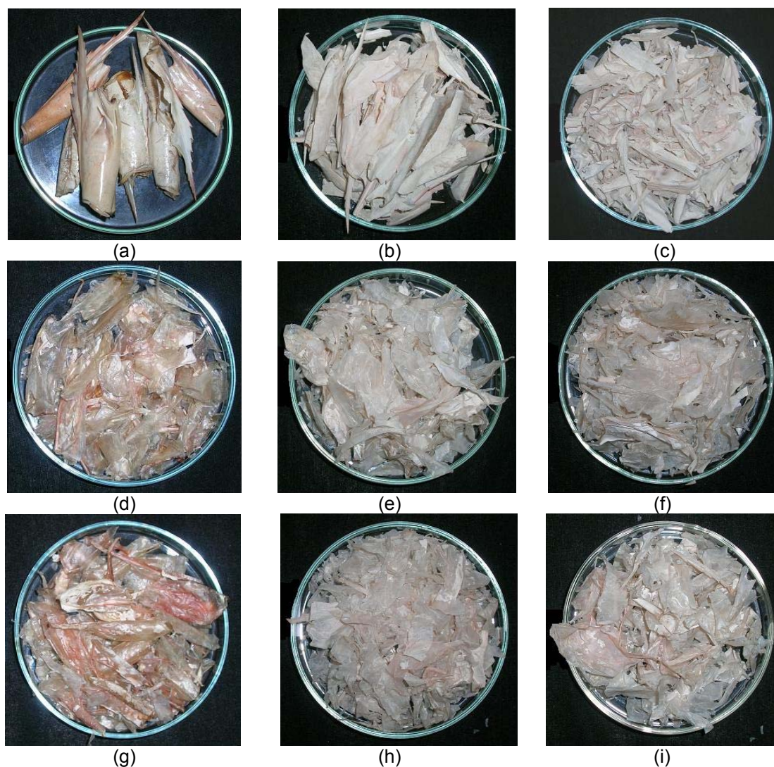
Fig 1. Appearance of chitin prepared under various deproteinization (DP) and demineralization (DM) times (a) DP/DM 0/0 (b) 15/0 (c) 30/0 (d) 0/15 (e) 15/15 (f) 30/15 (g) 0/30 (h) 15/30 (i) 30/30
