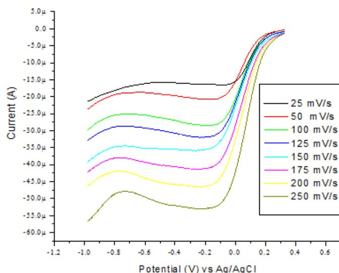
**Fig 6.** Linear sweep voltammogram signal of 5 mM Cr(VI) on SMZ-CPE with scan rate 25, 50, 100, 125, 150, 175, 200, and 250 mV/s in 0.3 M HNO<sub>3</sub>
