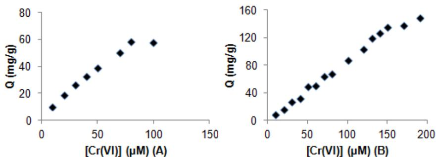
Fig 1. Chromate anion-exchange on (A) natural zeolite and (B) HDTMABr modified zeolite
