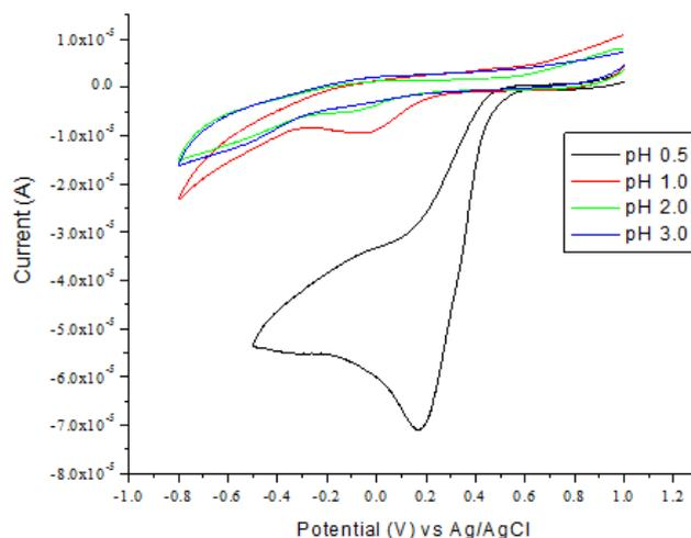
**Fig 4.** Cyclic voltammogram for reduction 13 mM at pH values of 0.5, 1, 2, and 3 on SMZ-CPE and with scan rate 100 mV/s
