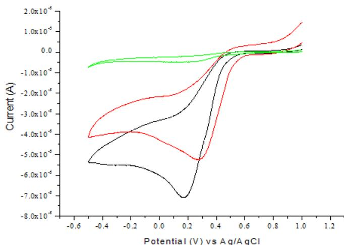
**Fig 3.** Cyclic voltammogram of 13 mM Cr(VI) in HNO<sub>3</sub> 0.3 M using CPE (—), SMZ-CPE (—), and gold electrode (—)
