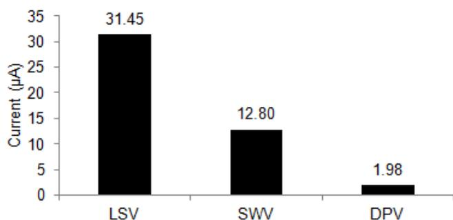
**Fig 5.** Measurement of 13 mM Cr(VI) using 3 different voltammetry techniques: linear swvp voltammetry (LSV), square wave voltammetry (SWV), and differential pulse voltammetry (DPV) on SMZ-CPE with scan rate 100 mV/s
