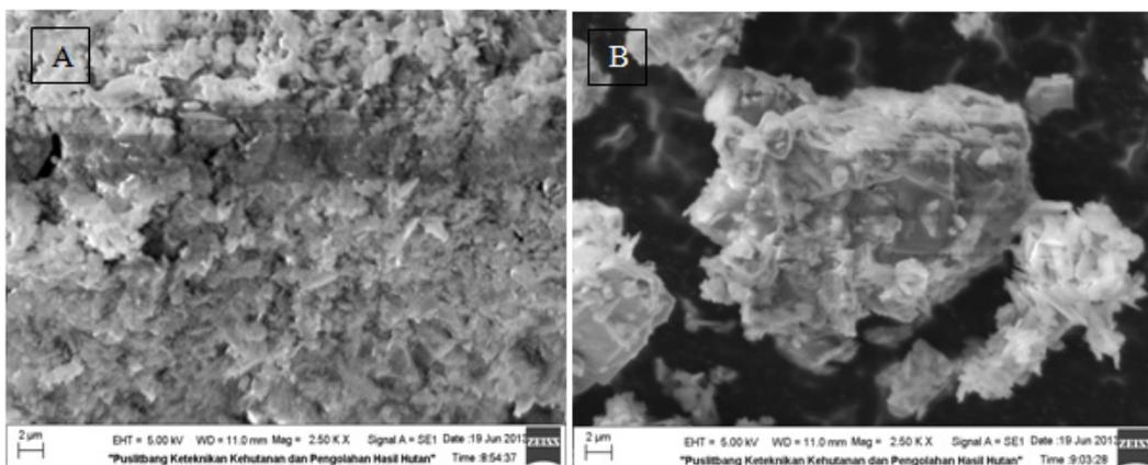
Fig 2. Photomicrograph of (A) natural zeolite and (B) HDTMABr modified zeolite
