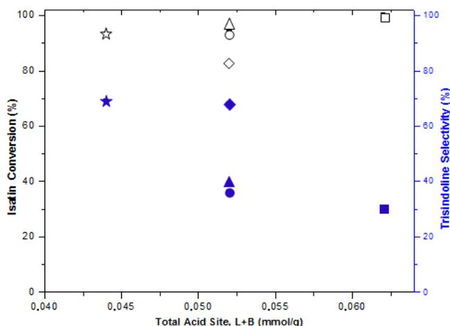
**Fig 7.** The relationship between the total acid sites on AM (☆), 1% AlCl<sub>3</sub>/AM (○), 5% AlCl<sub>3</sub>/AM (Δ), 10% AlCl<sub>3</sub>/AM (◇) and 15% AlCl<sub>3</sub>/AM (□) and the conversion of isatin (open) and trisindoline selectivity (closed)
