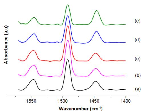
**Fig 4.** FTIR spectra of catalysts after being used in pyridine adsorption: (a) AM; (b) 1% AlCl<sub>3</sub>/AM; (c) 5% AlCl<sub>3</sub>/AM; (d) 10% AlCl<sub>3</sub>/AM; (e) 15% AlCl<sub>3</sub>/AM
