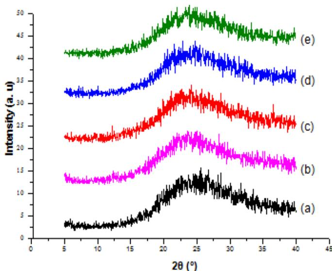
**Fig 1.** XRD patterns of catalysts: (a) AM; (b) 1%  $\text{AlCl}_3/\text{AM}$ ; (c) 5%  $\text{AlCl}_3/\text{AM}$ ; (d) 10%  $\text{AlCl}_3/\text{AM}$ ; (e) 15%  $\text{AlCl}_3/\text{AM}$
