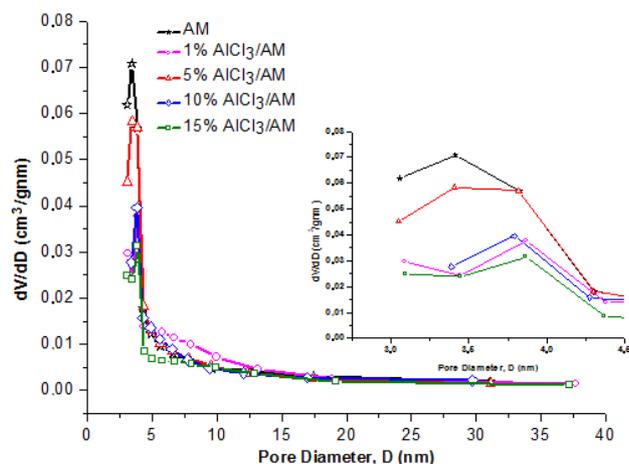
**Fig 6.** Pore size distribution (BJH desorption) of the catalyst
