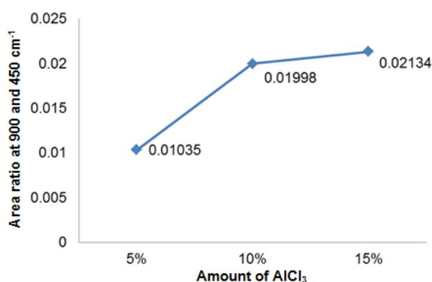
**Fig 3.** The effect of AlCl<sub>3</sub> amount to the area ratio at 900 and 450 cm<sup>-1</sup>
