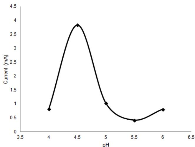
**Fig 4.** The current curve of the GOx/MCPE at pH 4.0-6.0, scan rate  $100 \text{ mVs}^{-1}$ . Cell conditions: 100 mM acetate buffer, 250 mM glucose, room temperature, 100 mM  $\text{K}[\text{Fe}(\text{CN})_6]$
