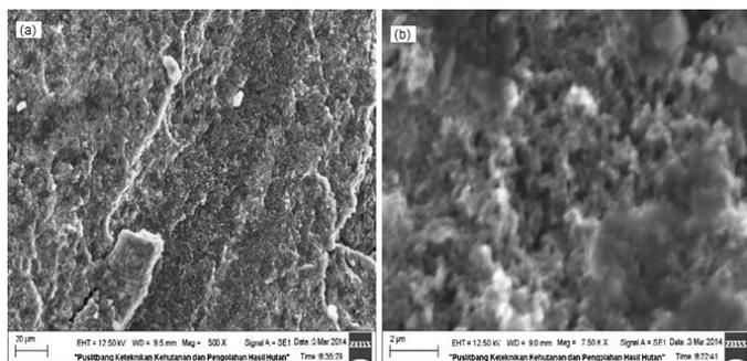
**Fig 2.** Polyaniline morphology by SEM with (a) 500 and (b) 7500 times magnification
