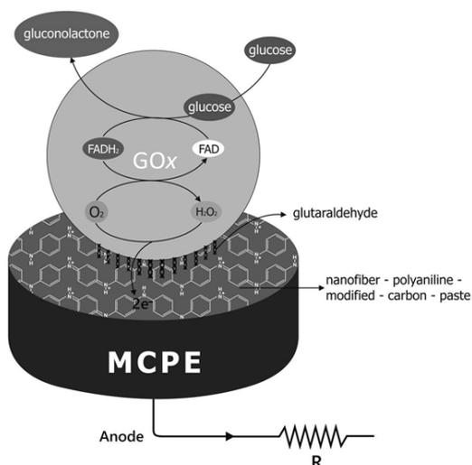
**Fig 1.** Schematic representation of the assembled GOx bioanode with nanofiber-polyaniline-modified-carbon-paste as an electron mediator
