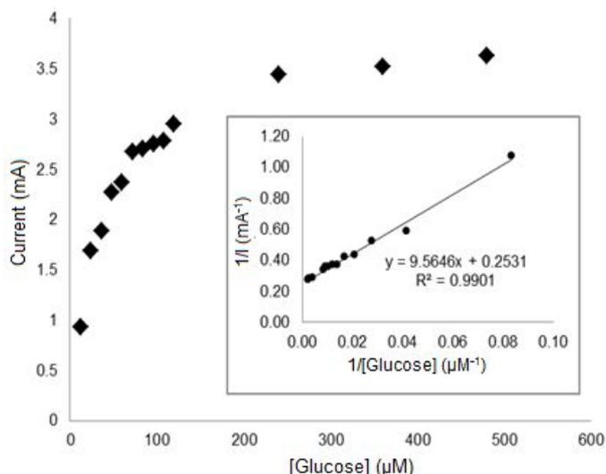
Fig 7. The current curve of the GOx/MCPE in the presence of various glucose concentrations in the electrolyte (range of 0.2 to 0.8 mM), scan rate  $100 \text{ mVs}^{-1}$ . Cell conditions: 0.1 M acetate buffer (pH 4.5), room temperature, 0.1 M  $\text{K}[\text{Fe}(\text{CN})_6]$
