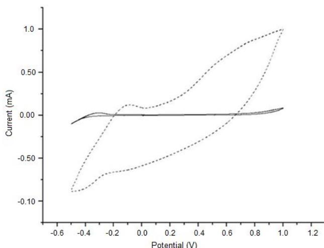
**Fig 3.** Cyclic voltammograms of CPE (black line) and MCPE (dashed line) at scan rate  $100 \text{ mVs}^{-1}$ , Ag/AgCl as reference electrode, cell conditions: 100 mM acetate buffer, 250 mM glucose, room temperature, 100 mM  $\text{K}[\text{Fe}(\text{CN})_6]$
