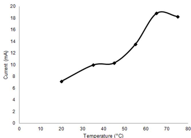
**Fig 5.** The current curve of the GOx/MCPE at temperature 20-80 °C, scan rate  $100 \text{ mVs}^{-1}$ . Cell conditions: 100 mM acetate buffer (pH 4.5), 200 mM glucose, 100 mM  $\text{K}[\text{Fe}(\text{CN})_6]$
