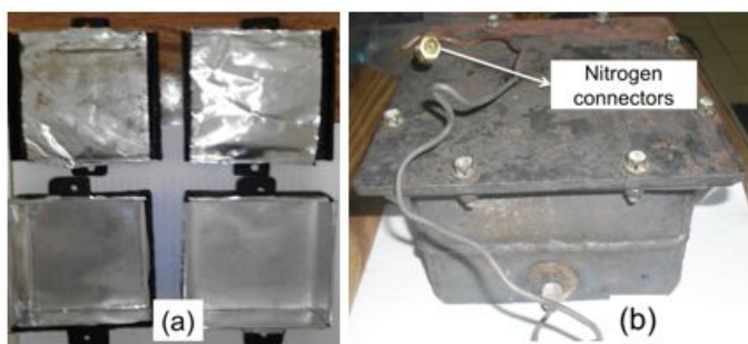
Fig 1. Synthesis equipments of carbon foam (a) mold coated by aluminum sheet (b) pyrolysis reactor
