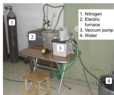
Fig 2. Instrumentation scheme of carbon foam synthesis
