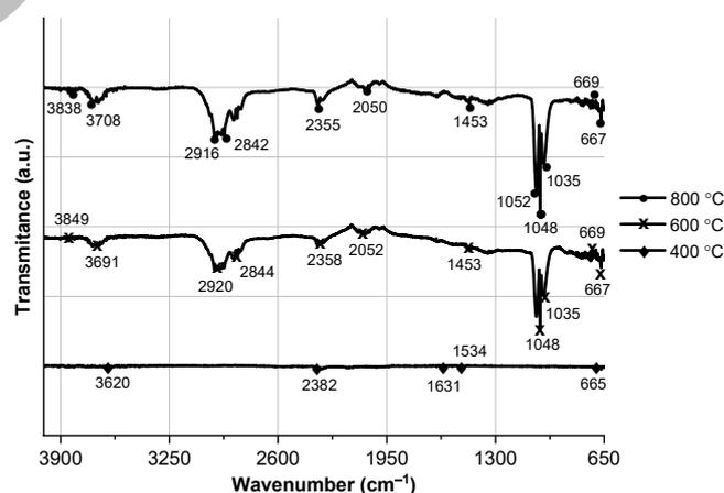
Fig 6. Graph of FTIR results of PKS after carbonization
