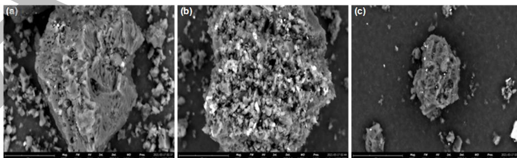
Fig 7. Microstructural SEM images of the activated PKS at (a) 400, (b) 600, (c) 800 °C activated temperature
