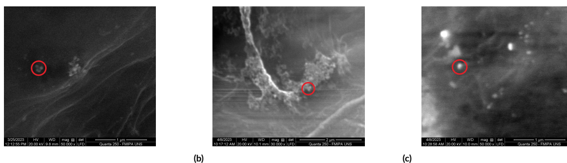
FIGURE 4 Scanning Electron Microscopy (SEM) image of surface morphology of silver nanoparticles at 50,000 \times magnification on filter paper pores, (a, b, c) silver nanoparticles extract 0.5%, 1.0%, and 1.5% respectively. Note: red circle indicates AgNPs.
