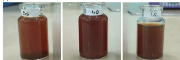
FIGURE 1 The color of the silver nanoparticle synthesis solution with various concentrations of S. jamaicensis leaf extract (0.5%, 1.0%, and 1.5%) at (a) 0 hours, (b) 24 hours, and (c) 48 hours.
