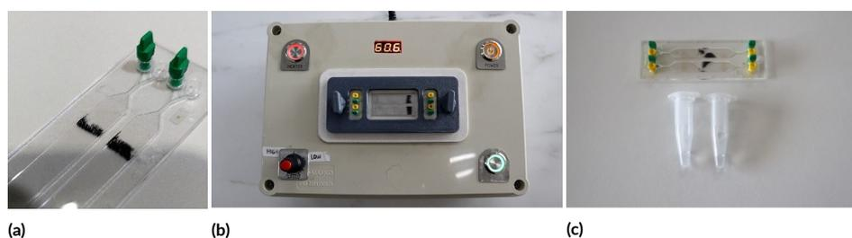
**FIGURE 5** Extraction process: (a) preparation of master mix together with magnetic beads in the chip; (b) the chip seated in the portable extraction unit with ChipGenie buffer at 60 °C; (c) result of extracted DNA placed in a mini tube to be ready for the amplification process.
