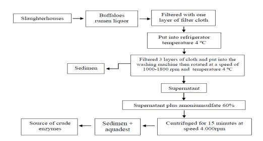
Figure 1. The cow rumen fluid extraction workflow from slaughterhouses, a modified use a washing machine (Budiansyah *et al.*, 2010).
