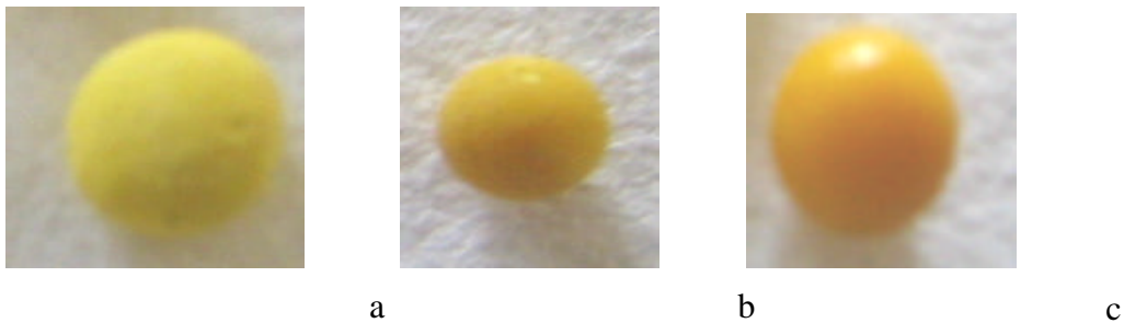
Gambar 1. Gel variasi medium (a) medium 2-etilheksanol, (b) medium \text{CCl}_4 , (c) medium minyak jarak kepyar
