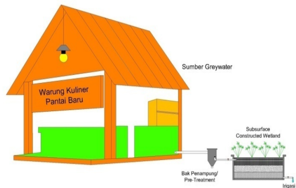
Figure 8. Sketch Using Greywater Management Unit Subsurface Constructed Wetland
