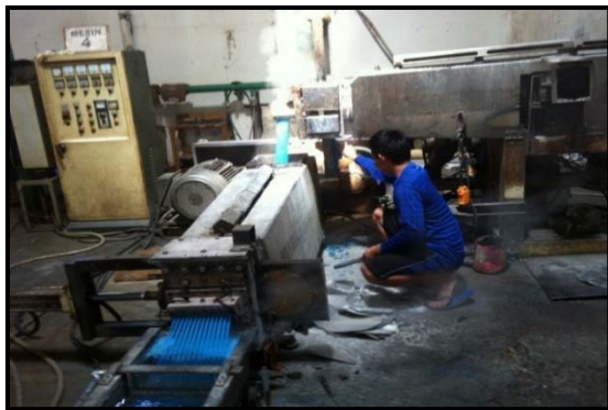
Figure 9. Pelletizing processing (Photo taking 31/07/2013)
