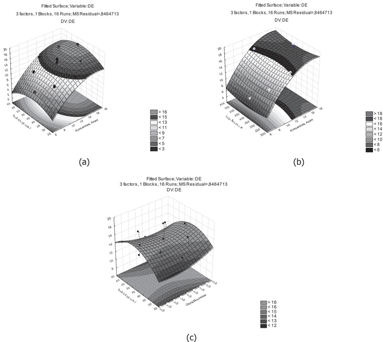
Figure 1. (a) Contour plot of RSM response surface on the effect of acetic acid concentration and liquefaction time on DE value; (b) Contour plot of RSM response on the effect of acetic acid concentration and microwave power on DE value; (c) Contour plot of RSM response surface on the effect of microwave power and liquefaction time on DE value
