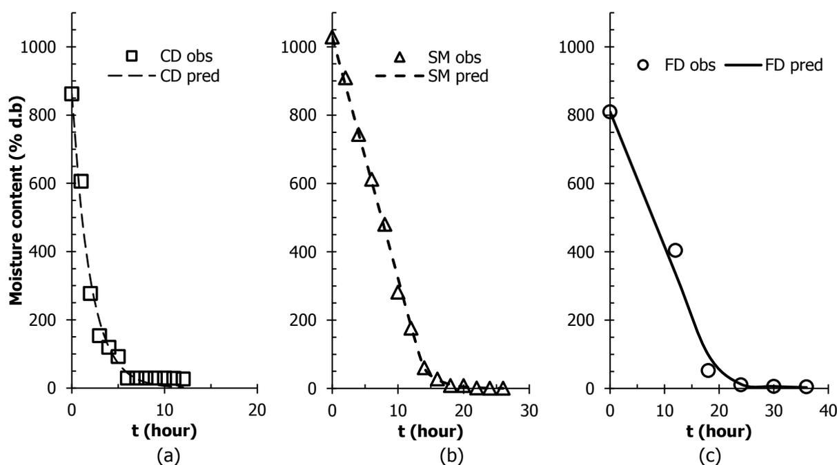
Figure 1. First-order kinetic of drying rose petals for Cabinet drying (CD) (a), Sunlight drying (SM) (b), and Freeze drying (FD) (c)
