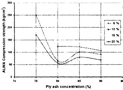
Figure 2. Compression strength vs. Fly Ash concentration
