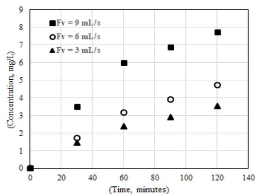
**Fig. 2:** The concentration of flavonoids extracted using different solvent flow rates as a function of time for the particle diameter of 4.01 mm.
