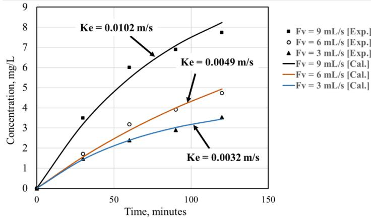
**Fig. 4:** Concentration of flavonoids as a function of time and solvent flow rate based on the calculation and experimental data for the particle diameter of 4.01 mm.
