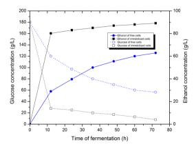
**Fig. 4**: Comparison of immobilized yeast and free cells system on glucose fermentation.
