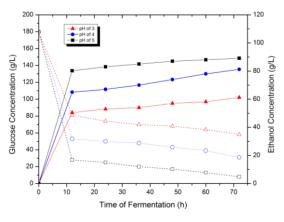
**Fig. 3**: The effects of pH medium on ethanol and glucose concentration
