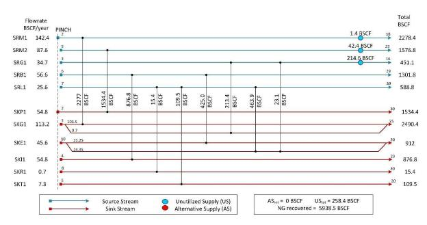
**Fig. 1**: The grid diagram of the natural gas network in a single region with a 0-year minimum time difference
