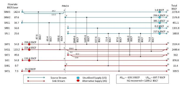
**Fig. 2**: The grid diagram of the natural gas network in a single region with a 3-year minimum time difference
