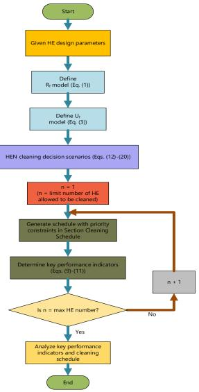
**Fig. 3:** Computation flowchart of cleaning scheduling for HEN
